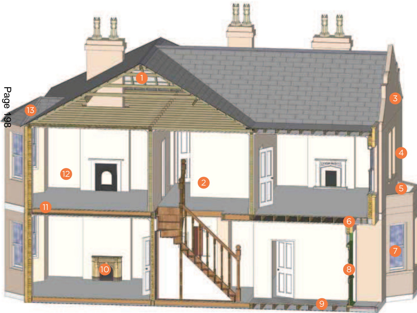
Section drawing of a typical Victorian/Edwardian house in Bath & North East Somerset
